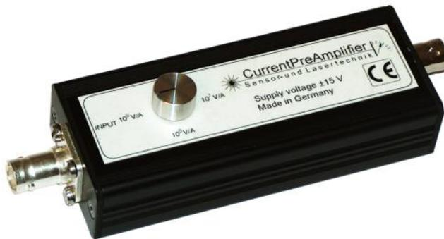
The amplification can be set by a 4-step switch: e.g.  $10^7 \dots 10^{10}$  V/A ; the bandwidth is switchable in two steps, 20Hz and 200 Hz. The detection limit depends on the amplification, the bandwidth and detector diameter. Please ask if you need other parameters
