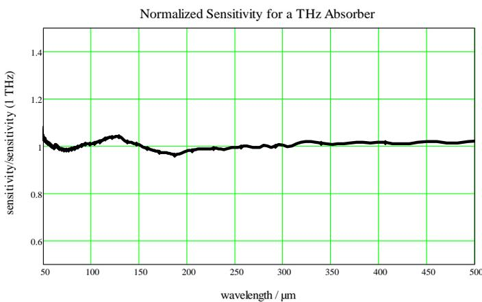
This figure shows the sensitivity of the pyroelectric detectors normalized with the sensitivity at 1 THz. Between 200 and 500  $\mu$ m the sensitivity changes within 2 %.
