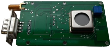
EMK200 with PEO12 sensor, DSUB9 connector
