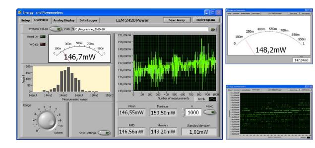
A Labview based software for displaying all via USB transferred data is also available. An overview window shows a small analog instrument, Histogram, data logger and also some statistical results. Additionally it is possible to save the showed data into a file.
